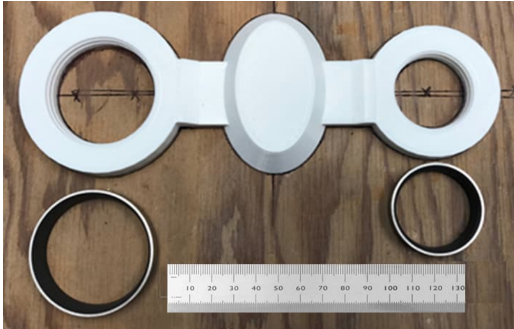
Figure 31. (a) A mold filling simulation for a 319 aluminum alloy in overcasting sand cavity simulated with sodium silicate bonded sand for three fill percentages showing the temperature distribution during filling and (b) the sand-casting pattern made of polylactic acid polymer with steel valve seats. Source: OSU
