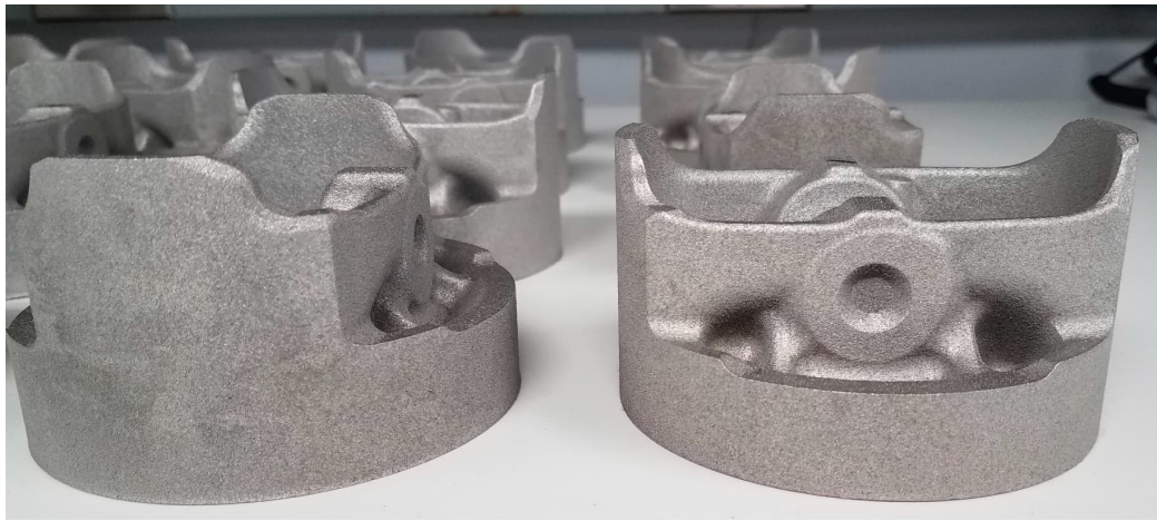
Figure 37. Additively manufactured pistons with an AlCeNiMnZr alloy. Source: ORNL.
