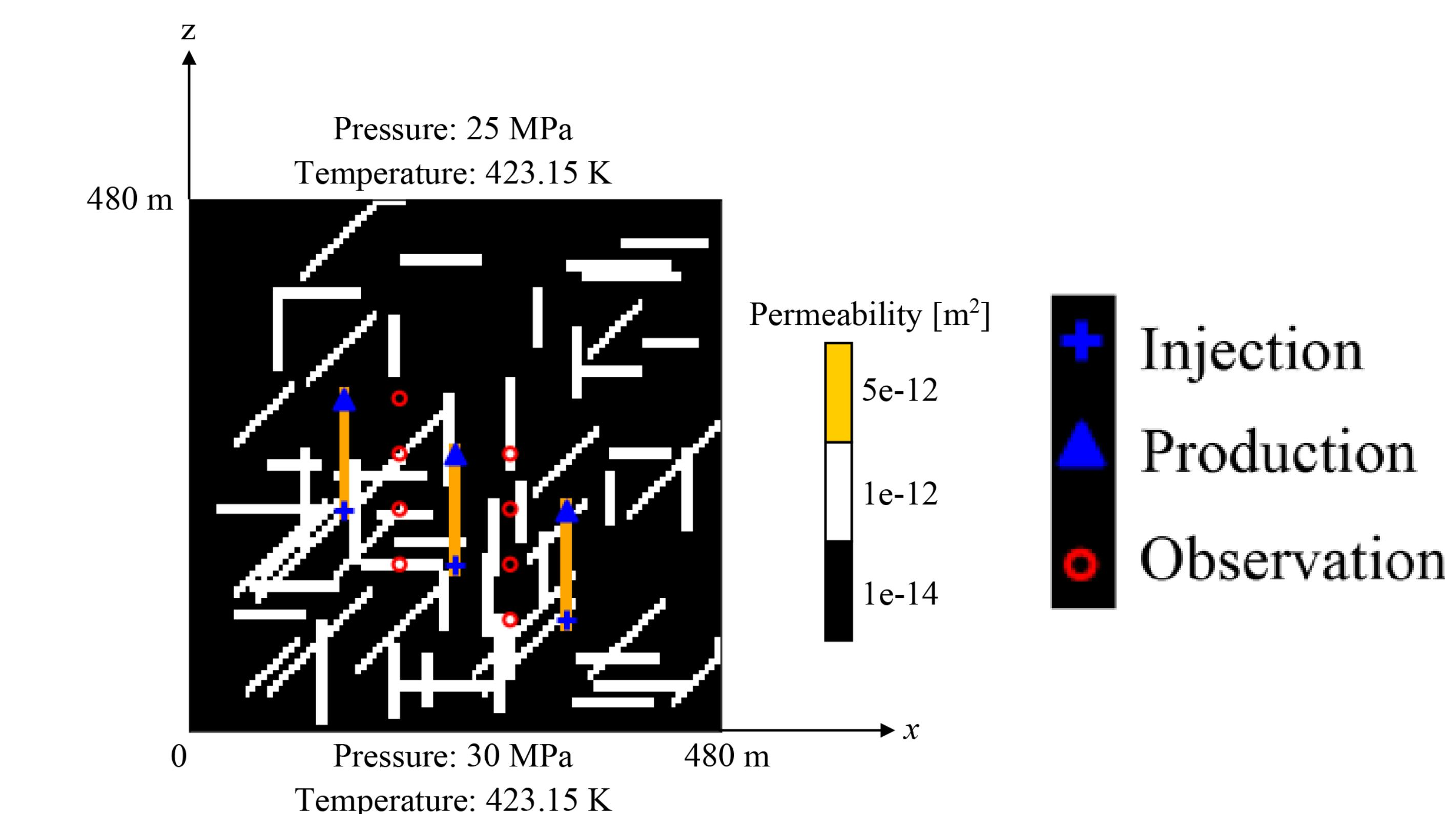
Three **line structures** (yellow lines) are determined as induced fractures by stimulations connecting the injection and production wells.
