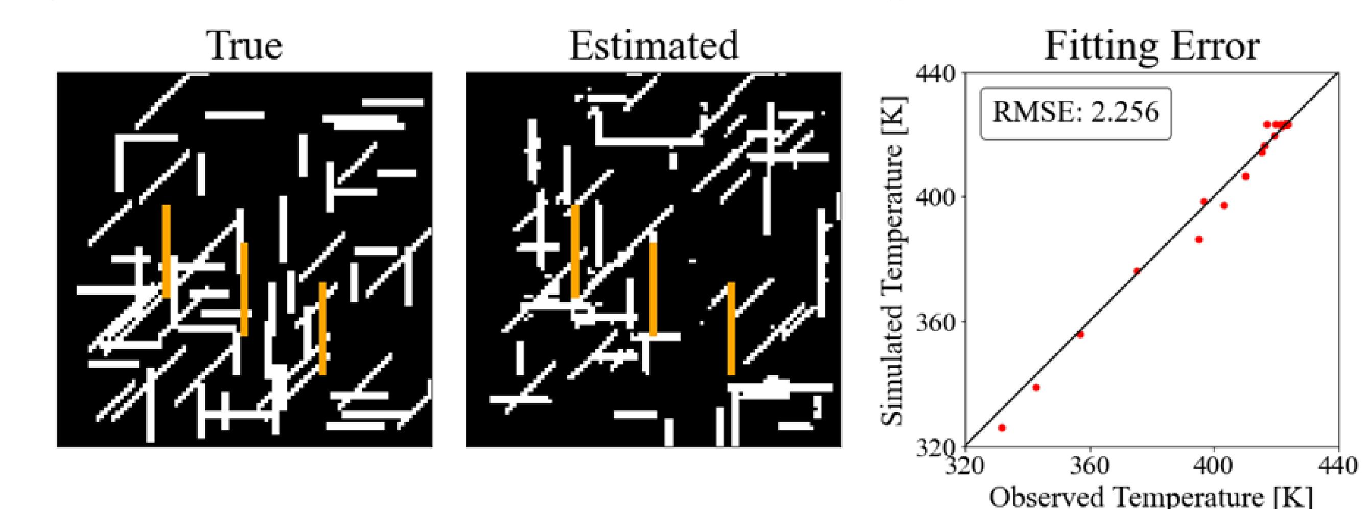
7-day simulation with 0.01  $m^3/s$  injection and production rates, temperature data were measured every day.
