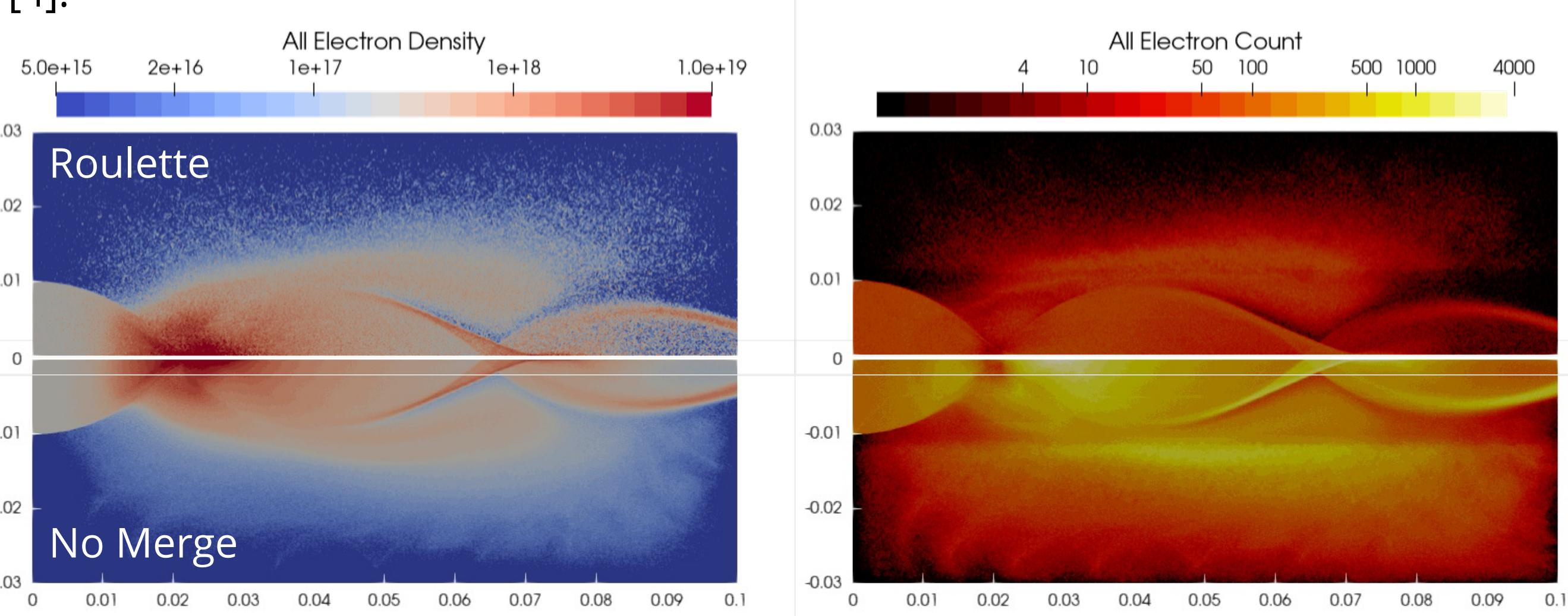
The Roulette Merge preserves important features although there is noise far from the symmetry plane and past the second pinch point. The number of particles per element is reduced significantly, in some cases from thousands to about one hundred. The number of particles at the second pinch point is a particular problem for the No Merge case; we can predict the location of the first and finely resolve the mesh there. Wall clock time is reduced by a factor of 4.7.
