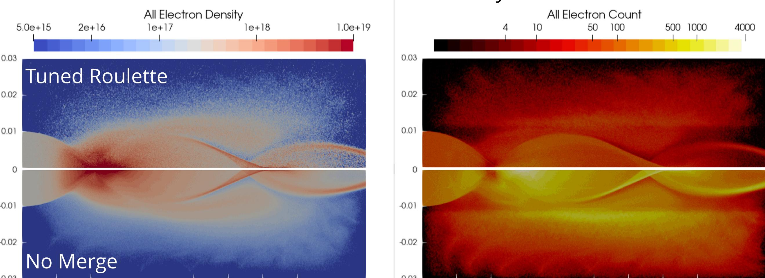
Tuning by distinguishing generations of electrons does not significantly affect the physical accuracy of the Roulette Merge. It is slightly less aggressive and there are more particles far from the symmetry plane. Wall clock time is still reduced by a factor of 4.1.
