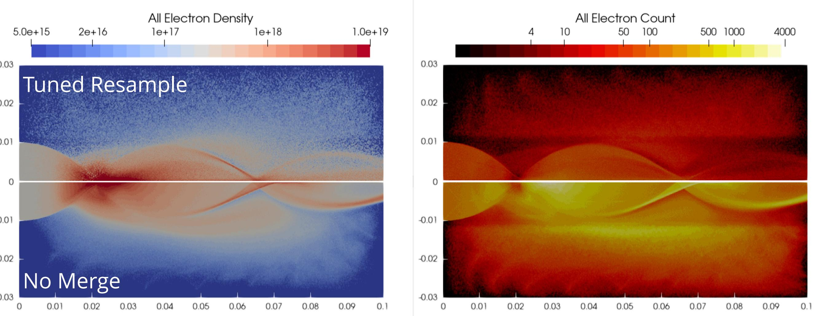
Tuning visibly improves the physical accuracy of the Distribution Resample Merge. The location of the second pinch point is more accurately reproduced, the secondary electron envelope above it is present although weaker than in the No Merge case, and the beam has a distinct though weak edge after the second pinch point. Wall clock time is reduced by a factor of 4.6.
