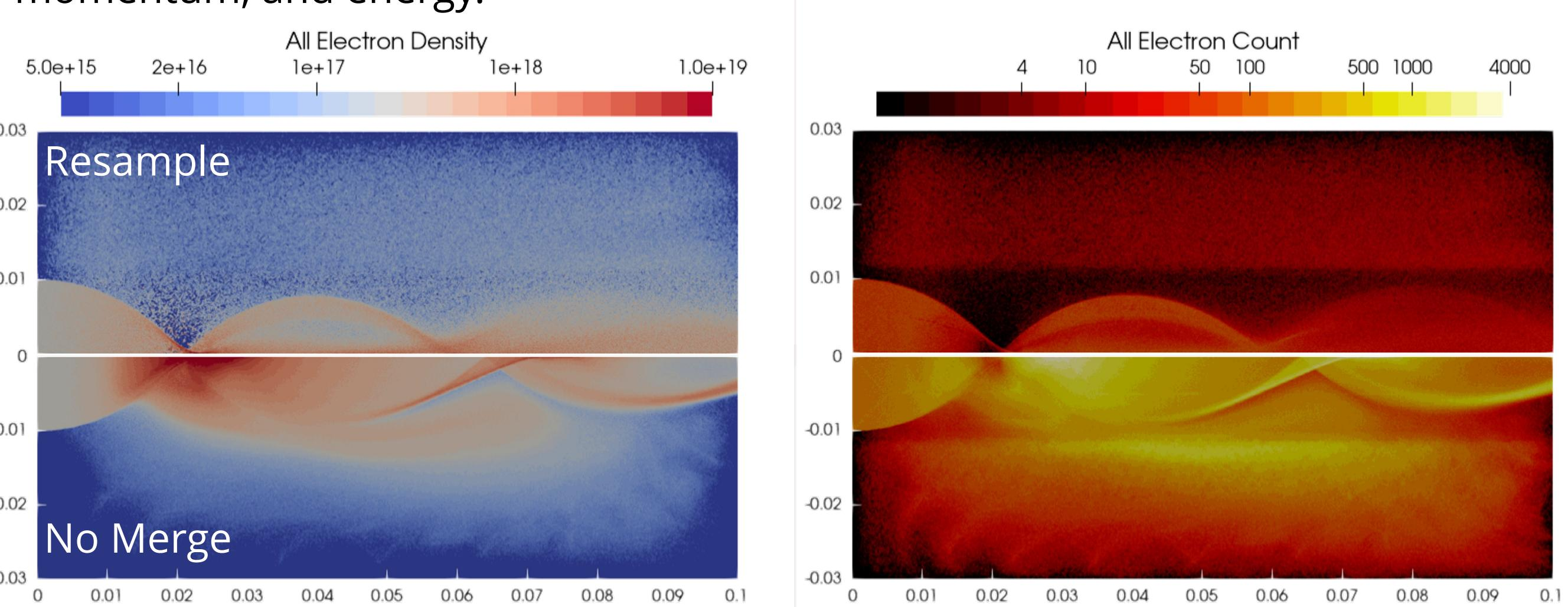
The Distribution Resample Merge fails to preserve important features such as the current density distribution on the right wall, and the second pinch point has moved, but the number of particles per element is significantly reduced. The merge struggles when asked to reduce the combined population of beam electrons and secondaries. Wall clock time is reduced by a factor of 3.8.
