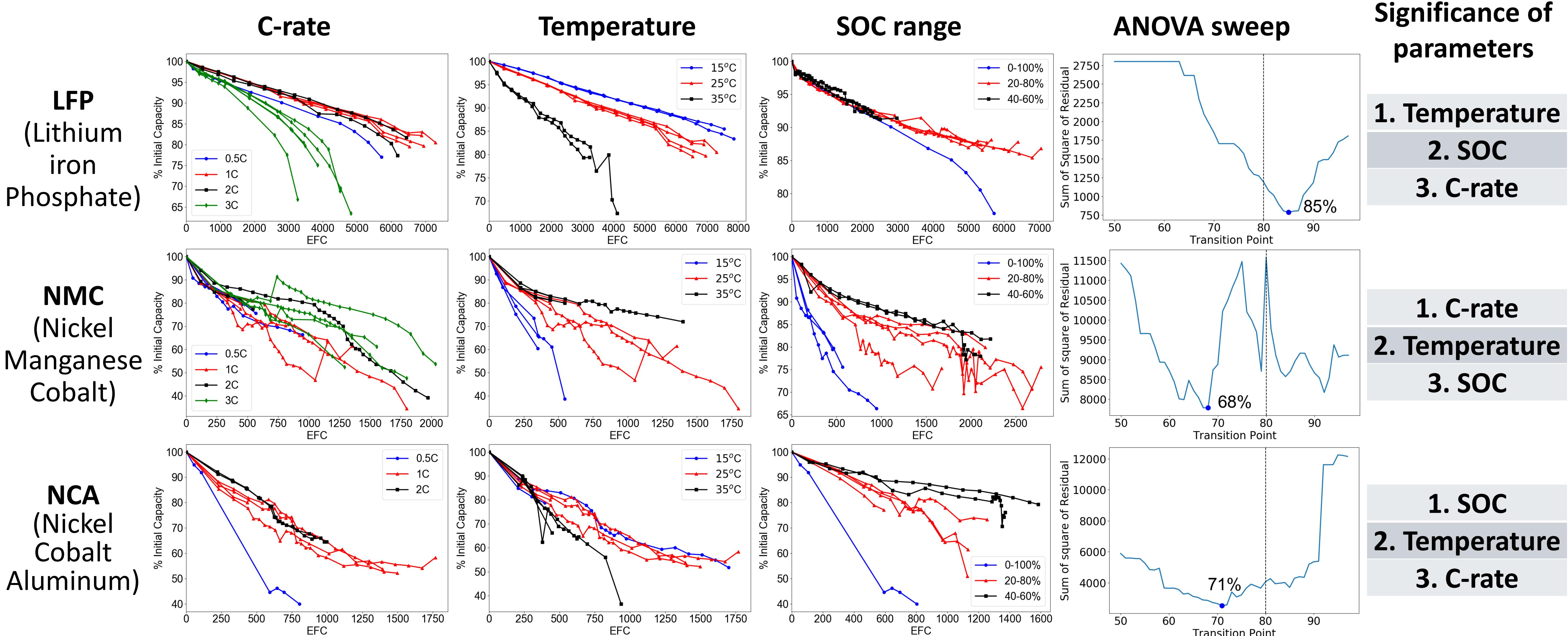
The point of change in degradation behavior varies based on chemistry and use conditions and is not necessarily 80%.
