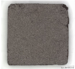
Casting of \text{Fe}_4\text{N} Plates
