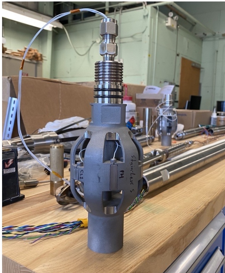
Figure 2-4: Fabricated sensor housing populated with installed sensors and bulkhead fitting.
