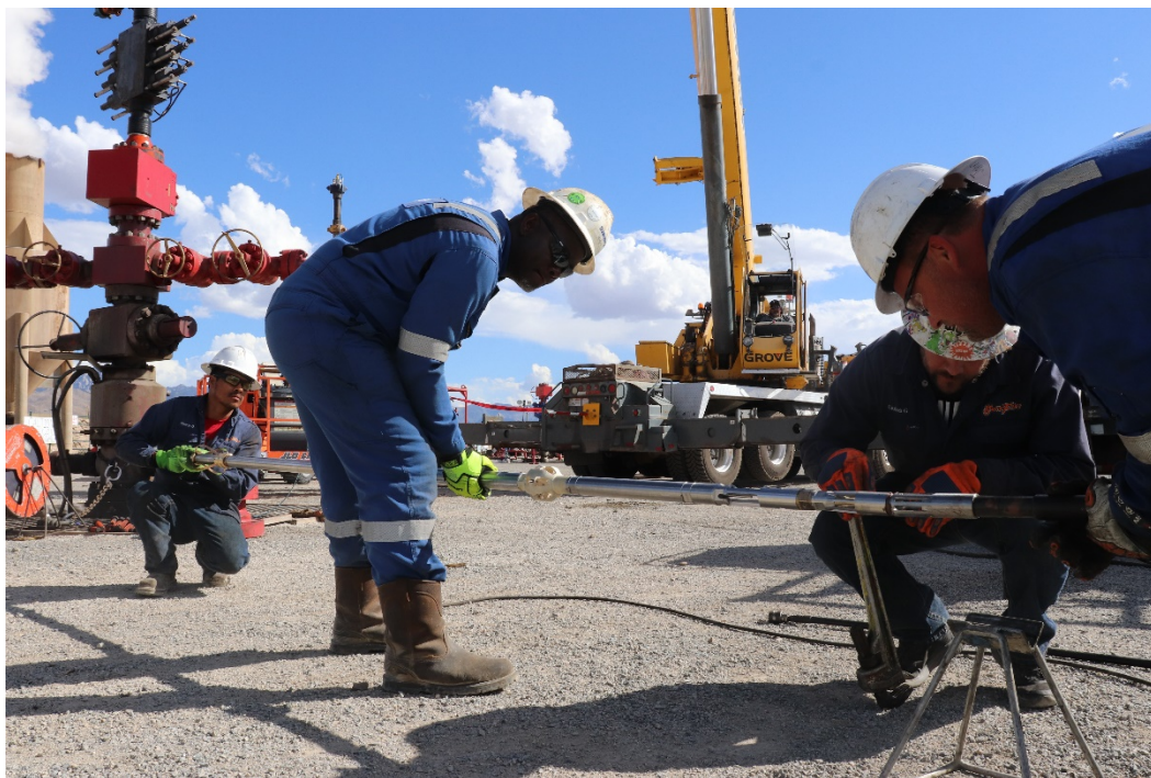
Figure 4-8: Full chemical tool assembly attached to weight bars and being loaded into lubricators.
