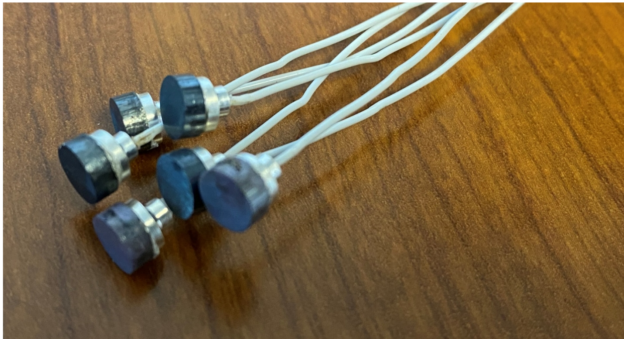
Figure 2-2: ISE and reference sensor assemblies before application of Gagekote.
