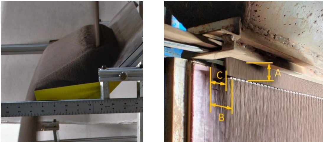
Figure 1. Multistage particle trough obstruction (left; G3P3-USA) and the perforated plate obstruction (right; G3P3-KSA)
