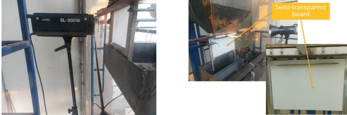
Figure 17. The DC lamp behind the PHR (left) and the semi-transparent PHR board seen from the front (right); only the back-side lamp was on during the opacity measurements.
