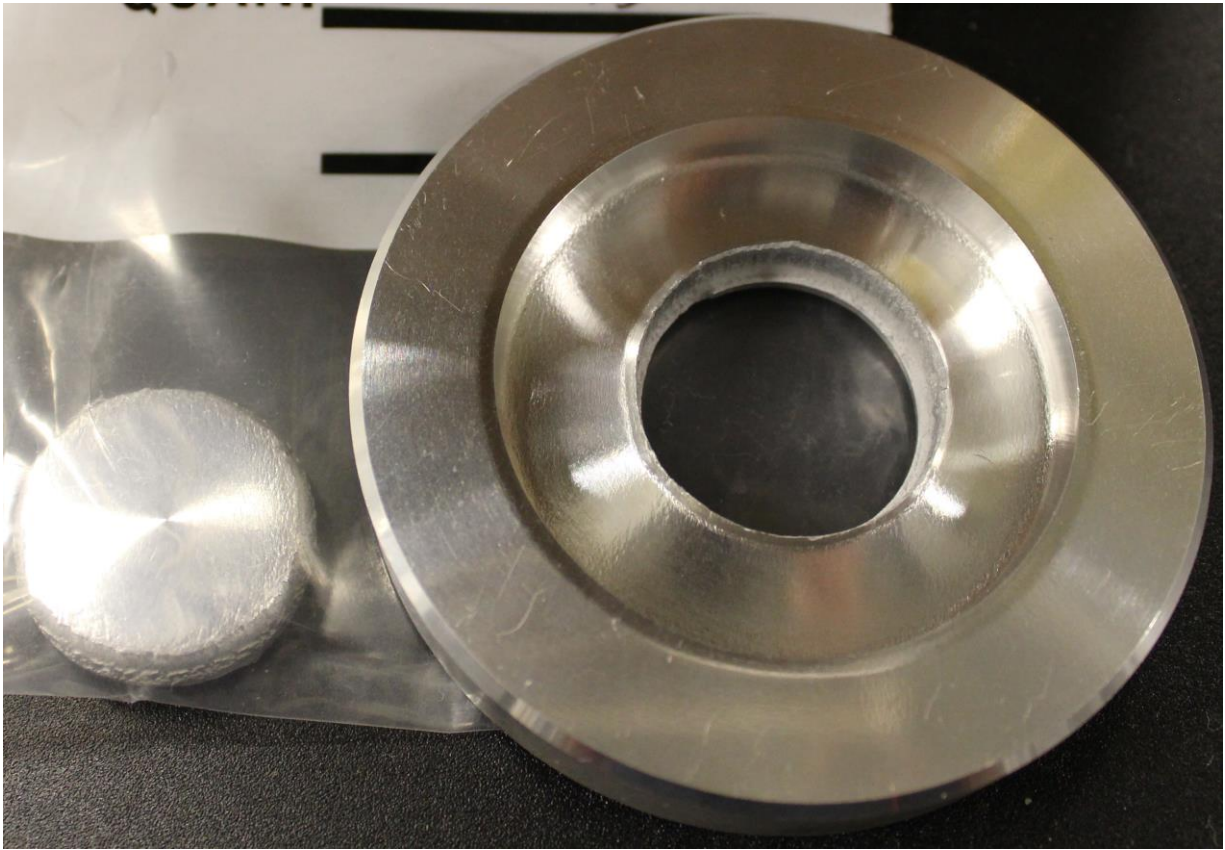
Figure 21: Specimen T250-15 and Ejected Plug After Test 102 with One-Inch Probe
