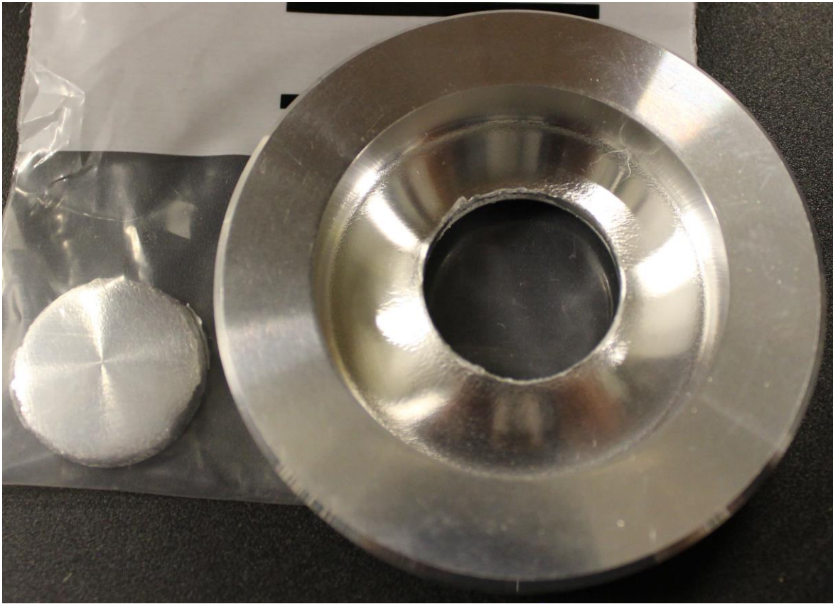
Figure 15: Specimen T125-12 and Ejected Plug After Test 65 with One-Inch Probe
