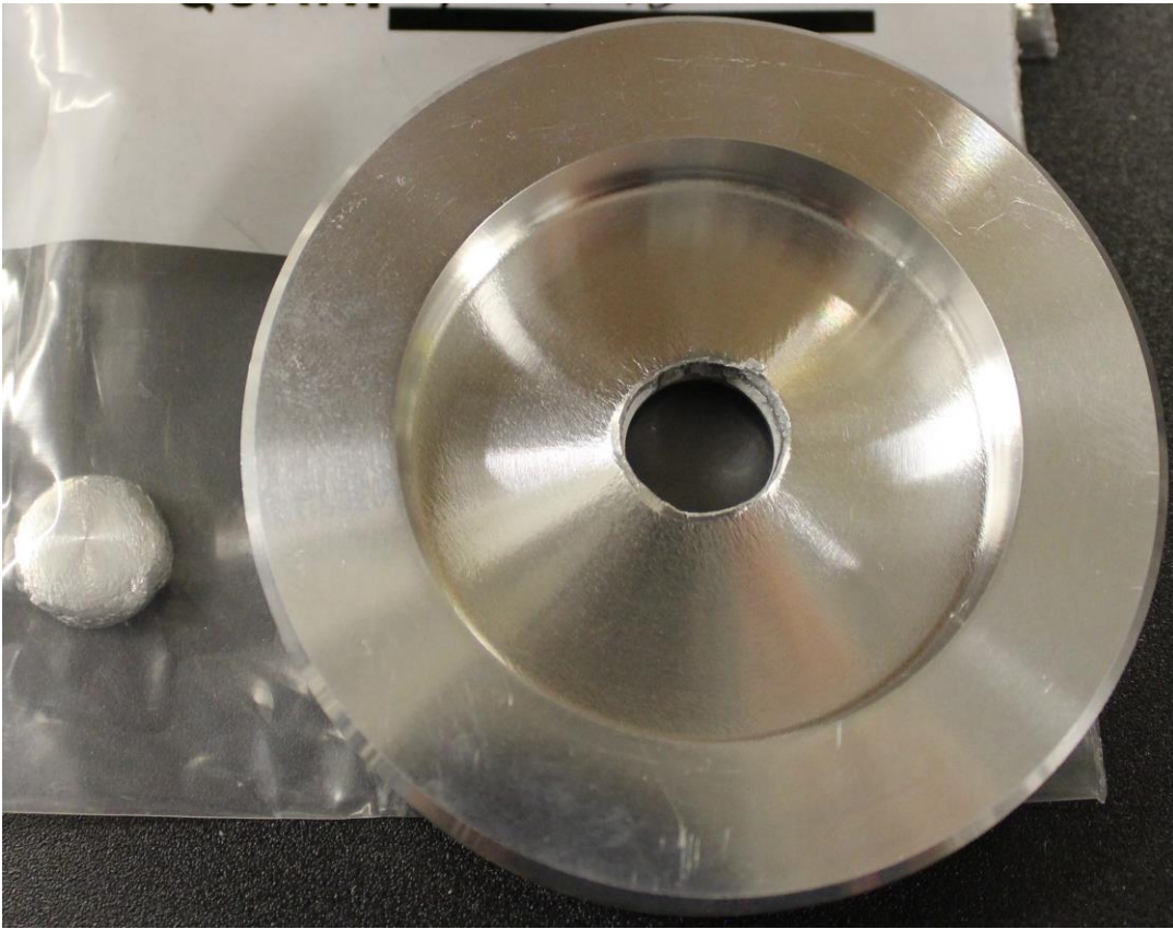
Figure 17: Specimen T188-09 and Ejected Plug After Test 81 with One-Half-Inch Probe
