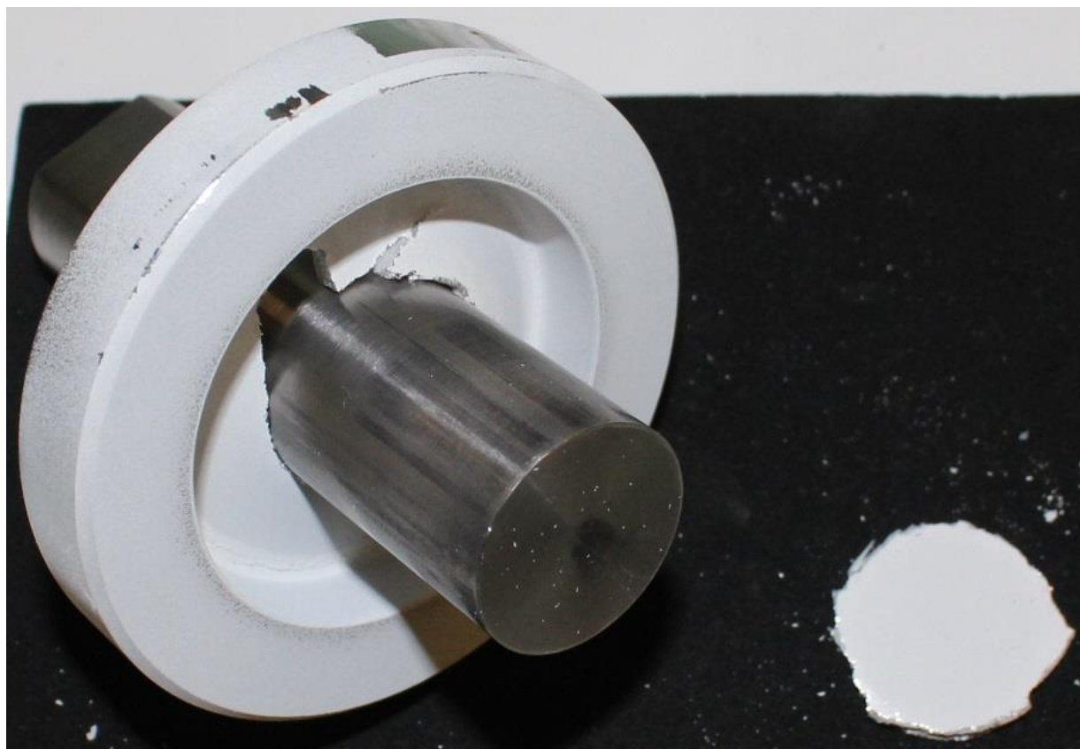
Figure 24: One-Inch Flat-End Probe Impaled In Specimen T114-14 After Test 52
