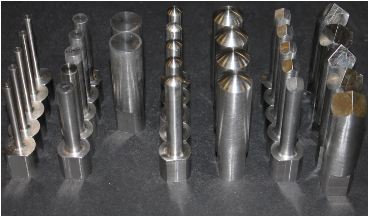
Figure 12: Flat-End, Spherical, and Tri-corner Probes of Various Diameters
