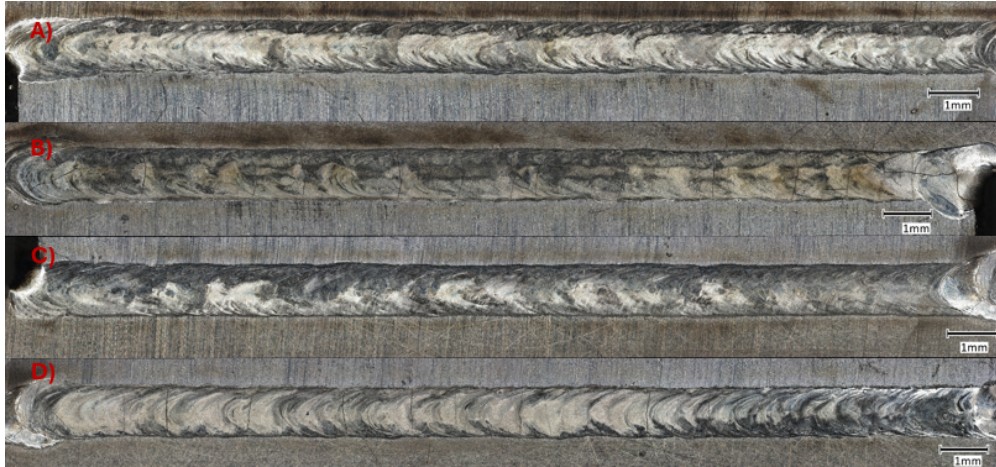
Figure 12: Matrix 3: A) 0.003" into Inconel 625 B) 0.003" into vanadium C) 0.004" into Inconel 625 D) 0.004" into vanadium
