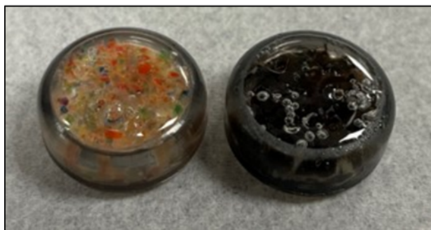
Figure 2: Two early Puck prototypes composed of 3D printed body, interior sensing mixture, and epoxy poured-in lid to provide an oxygen impermeable shell. (Left) Puck coupon without an intentional breach of air-tight outer shell (i.e., un-tampered); (Right) Puck coupon with an intentional breach of air-tight outer shell (i.e., after simulated tamper attack).
