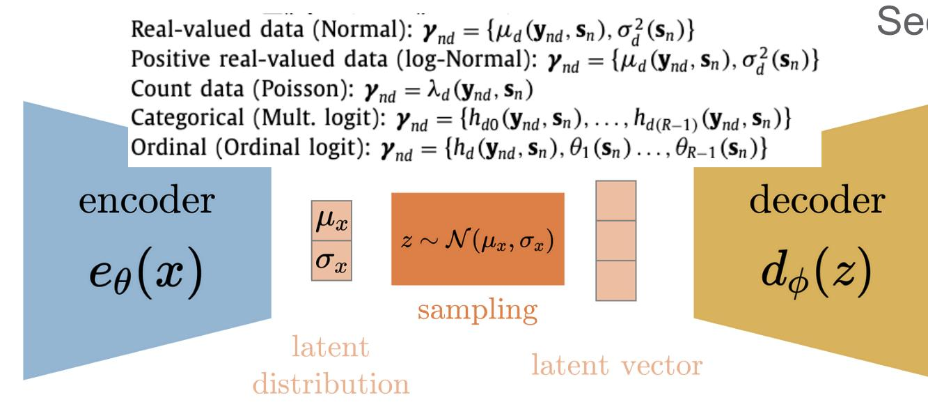
$$\text{reconstruction loss} = \|x - \hat{x}\|_2 = \|x - d_\phi(z)\|_2 = \|x - d_\phi(\mu_x + \sigma_x \epsilon)\|_2$$
