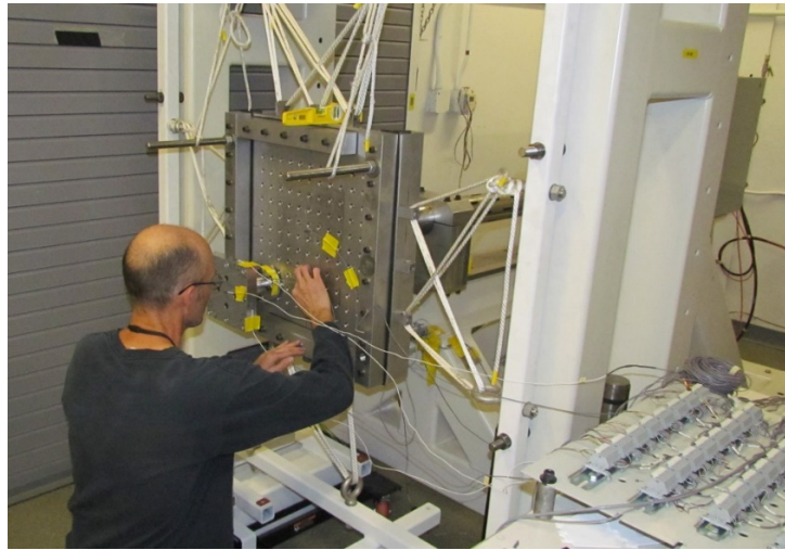
Figure 1: Preparation of a resonant plate for shock testing. The plate is suspended by rope. A test article can be attached to the front of the plate. The air gun is visible behind the plate.
