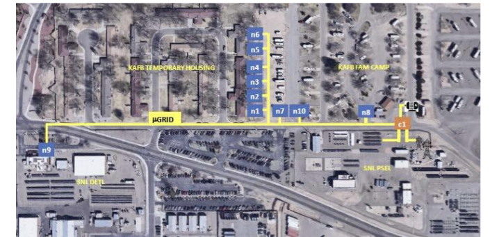
Ten-node BlockEnergy Microgrid on Kirtland Air Force Base
