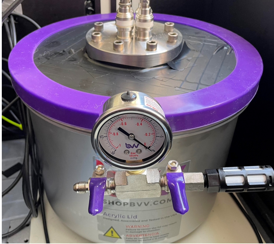
Figure 1: Vacuum chamber used for OCT measurement.
