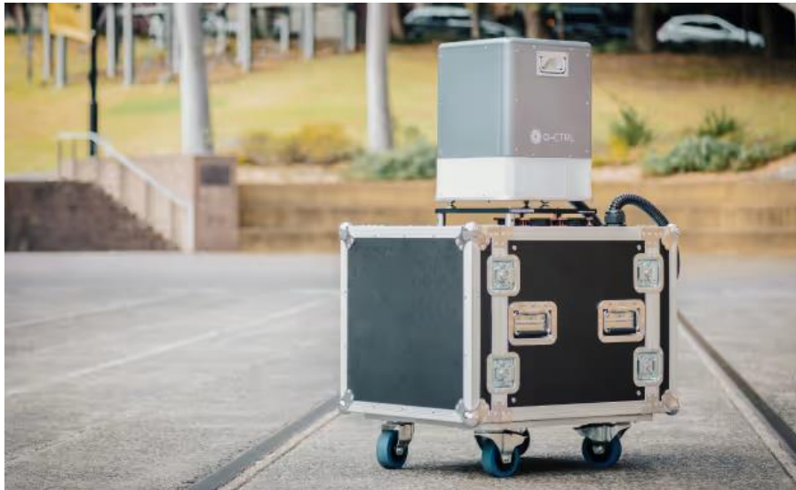
Figure 2. Picture depicting Q-CTRL's compact, 3-axis quantum IMU. 68
