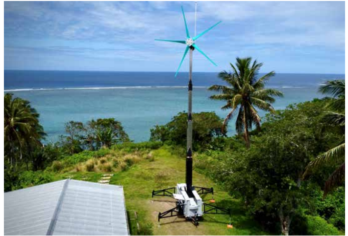
Shown deployed in a remote coastal location, this Uprise Energy Mobile Power Station was set up in minutes and began generating power immediately. Photo from Jonathan Knight, Uprise Energy
