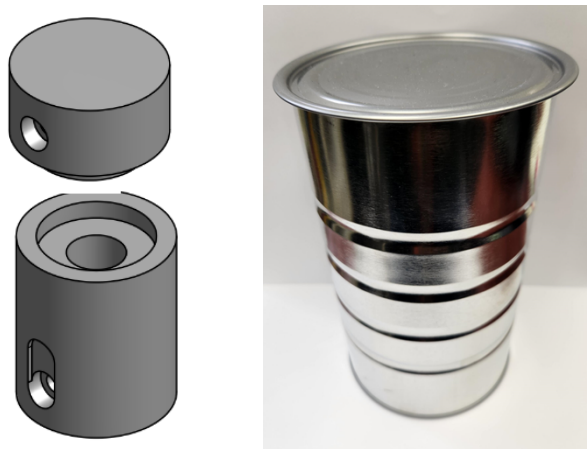
Figure 2. The current standard shipping container for ^{224}\text{Ra}/^{212}\text{Pb} generators. (left) Drawing of the 1.25 in. lead pig used for generator shipments. (right) Example of a can with crimp-style lid that is the standard for ^{224}\text{Ra}/^{212}\text{Pb} shipments. The original isotope cans have a pull tab at the bottom to open the can. The can shown here requires a can opener.
