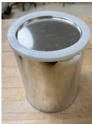
Figure 3. Picture of the paint-can-style Hazmatpac can shipping container with locking ring. This can was tested as a secondary shipping configuration for ^{224}\text{Ra}/^{212}\text{Pb} generators.
