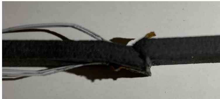
Figure 11: Failure of Compressive Specimen
