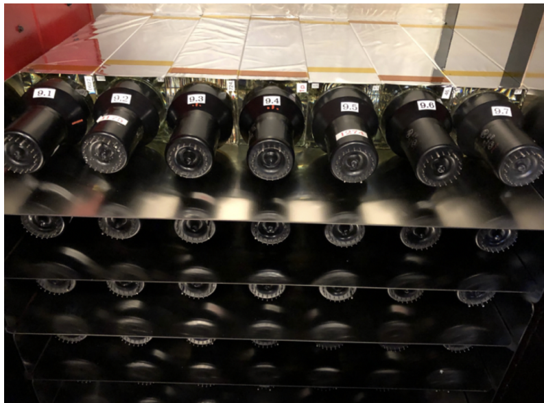
Figure 2.10: Lead-glass blocks stacked in the Shower. PMTs are attached to the lead-glass blocks which are stacked in the Shower housing. [35].
