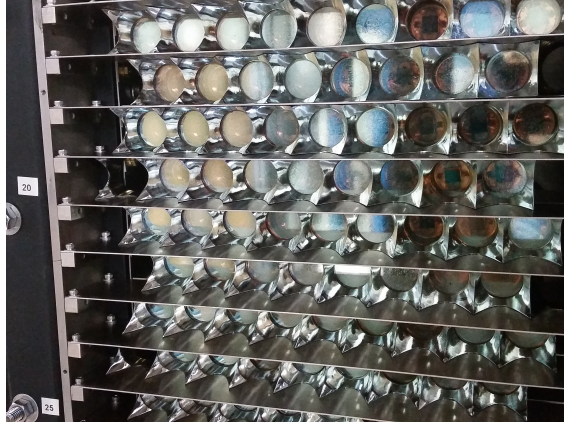
Figure 3.8: Photograph of a section of the GRINCH PMT array as seen from inside the detector. The aluminum-coated light-catchers focus the Cherenkov light onto the face of the PMTs in each cell.
