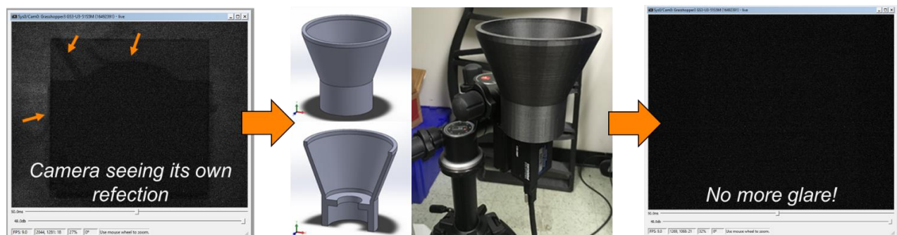
Figure 8. An image before (left) and after (right) the collar was added that shows significant glare reduction.
