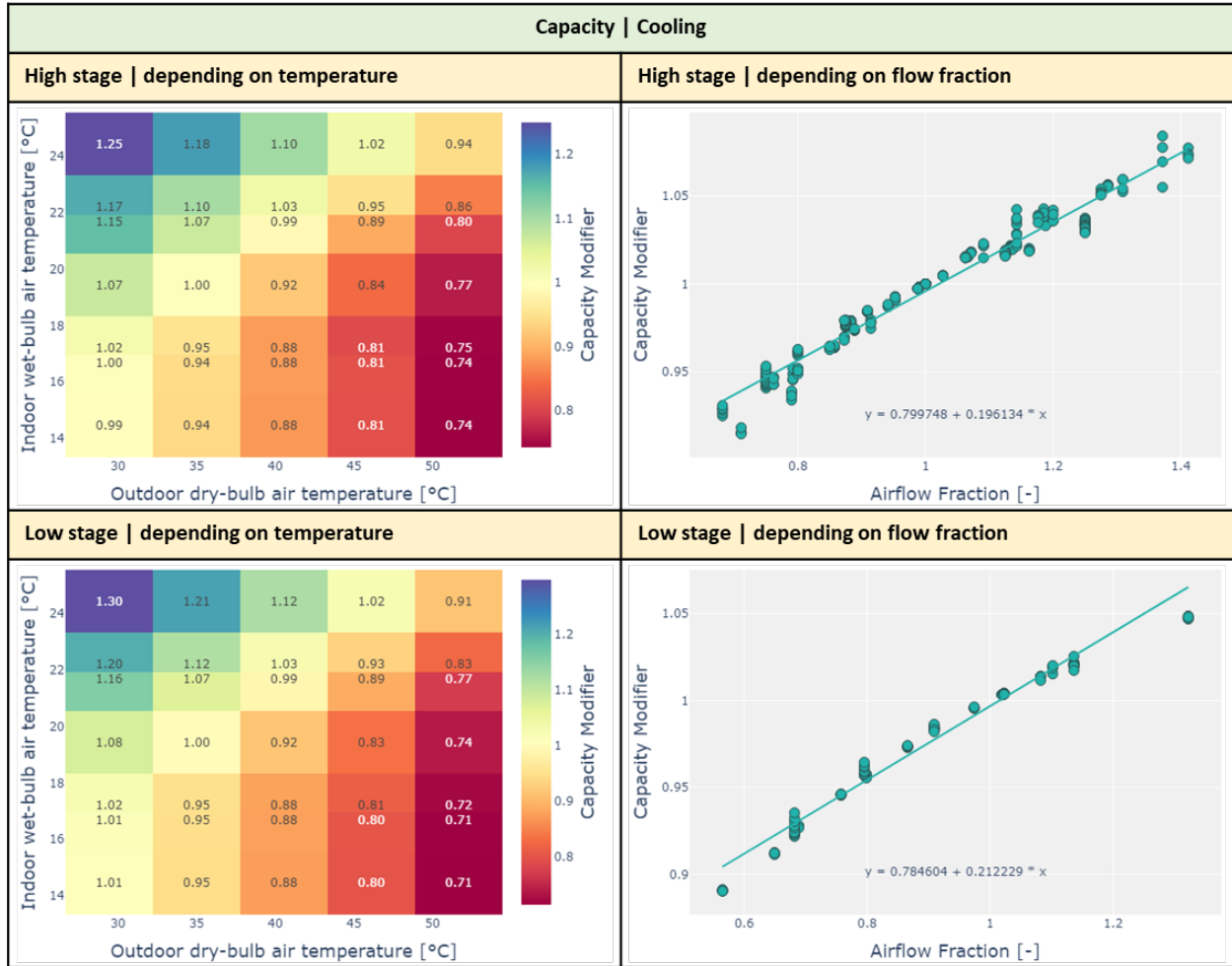
Figure 3. Averaging/fitting results of new performance maps: cooling capacity
