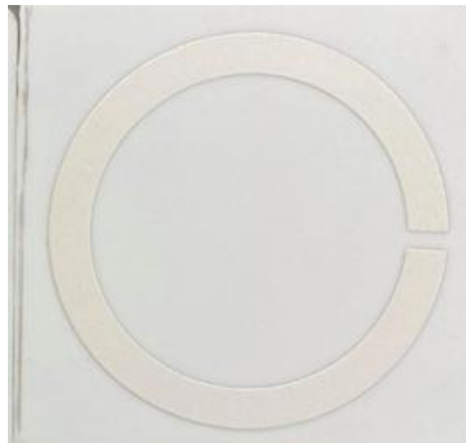
Split ring design printed on alumina substrate with silver ink
