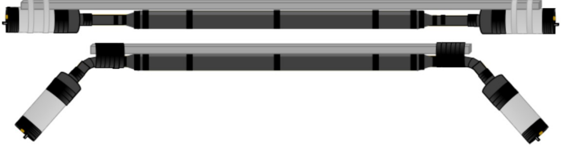
Figure 4.15: A diagram of the two types of scintillator bar assemblies, showing the light-tight scintillator bars, the light guides, the PMT housings, and support bars. Adapted from [132].
