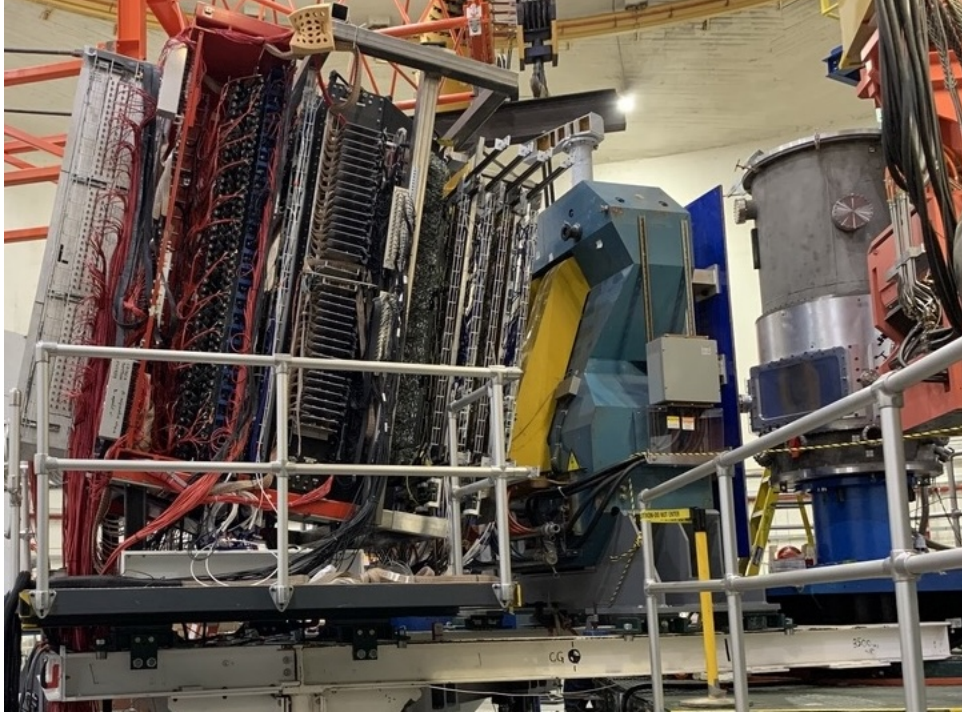
Figure 4.11: A picture of the BigBite Spectrometer in Hall A, with the target chamber on the right.
