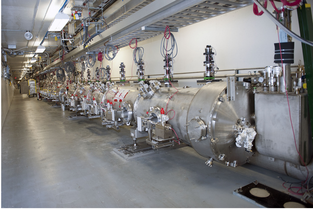
Figure 4.2: Two partially installed C-100 cryomodules.
