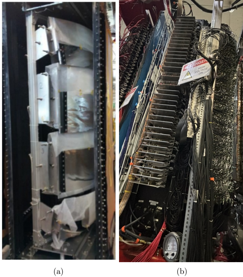
Figure 4.13: Left: The GRINCH from a side view showing the cylindrical mirrors. Right: A side view of the GRINCH installed in BigBite, taken from beam left, showing the PMT array and front-end NINO electronics.
