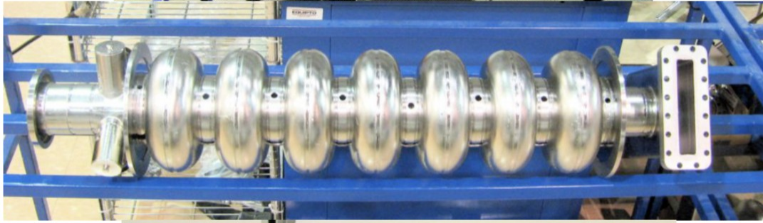
Figure 4.3: Seven-cell SRF Cavity. Adapted from [116].
