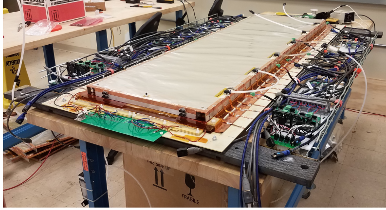
Figure 5.9: A UVA UV GEM layer. The layer is one single module with a 150 \times 40 \text{ cm}^2 active area. This layer has RF shielding instrumented, which is identical to how the GEMs of this type would have been installed in the BigBite Spectrometer.
