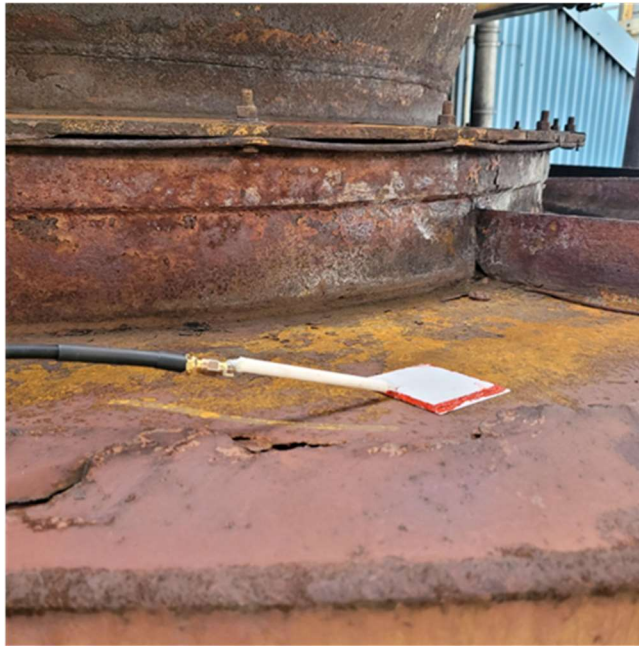
Figure 6.2: Picture of the packaged sensor with embedded interrogator antenna connected to a coaxial cable connected by an SMA connector to the nano-VNA (that is out of picture view).
