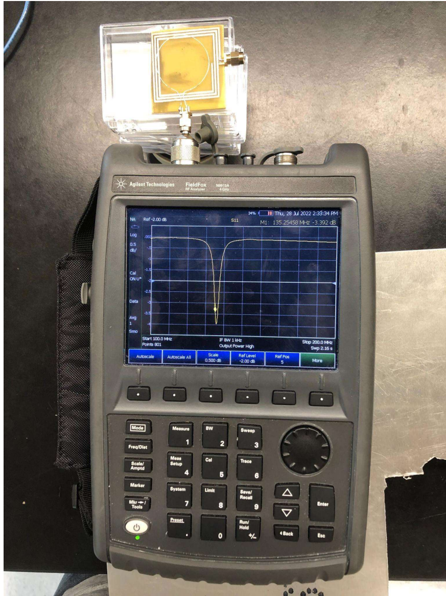
Figure 5.2: Measured S11 response of LC sensor through air.
