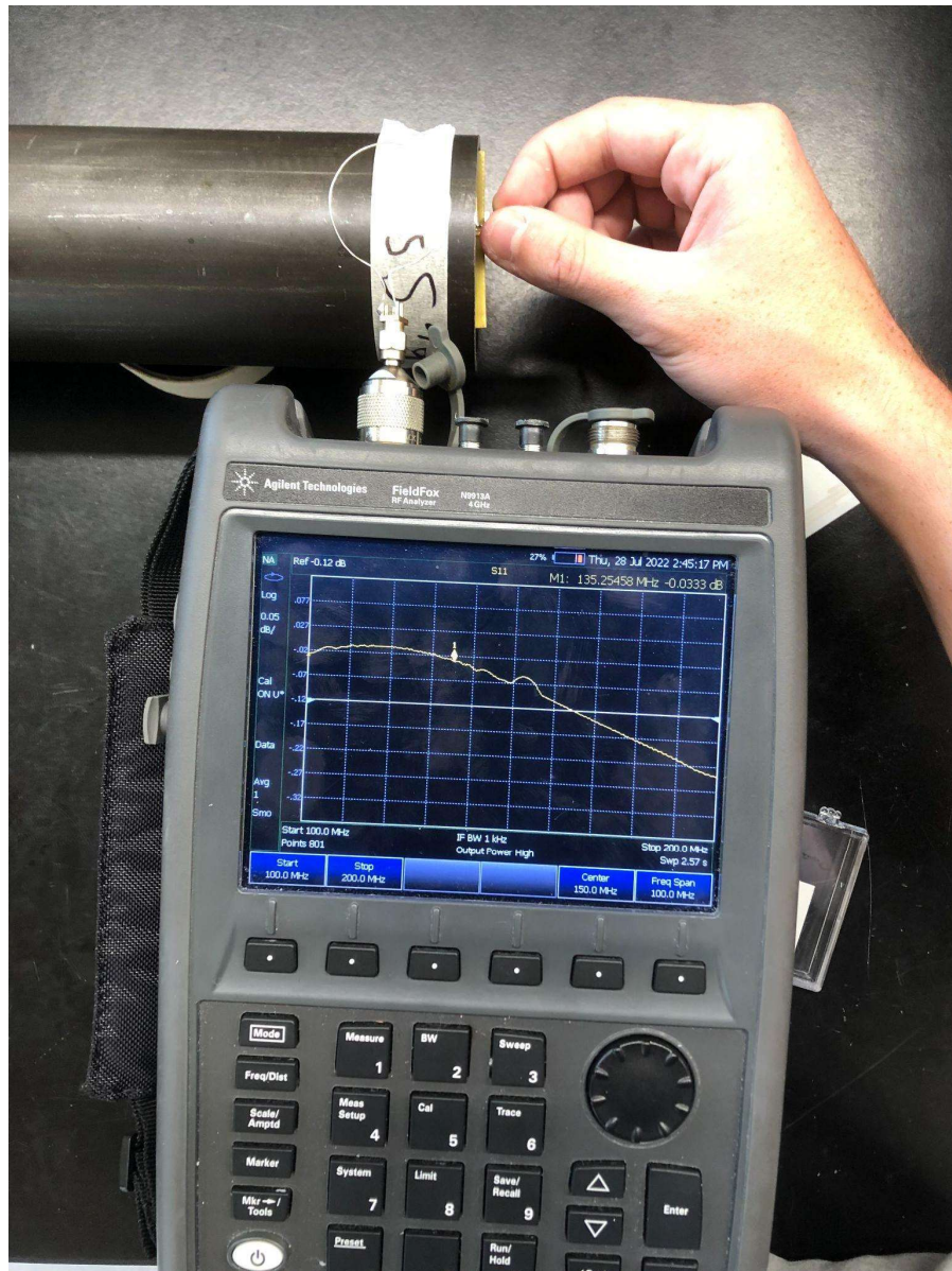
Figure 5.3: Measured S11 response of LC sensor through stainless steel.
