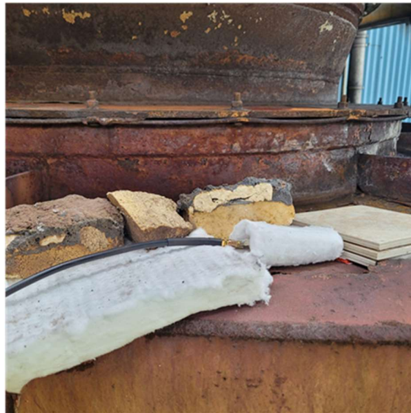
Figure 6.3: Picture of sensor embedded under ceramic tiles to protect against the weather elements, and alumina fiber insulation to protect the coaxial cable from touching the metal cyclone surface (insulation brick pieces just used to hold all parts from moving due to wind).
