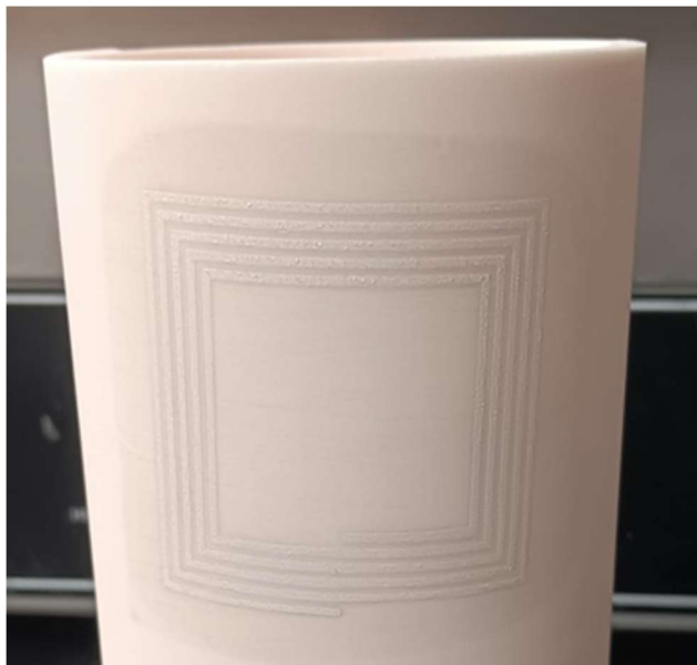
Figure 3.11: Peel and stick process sintered Ag on curvature Al 2 O 3 substrate.
