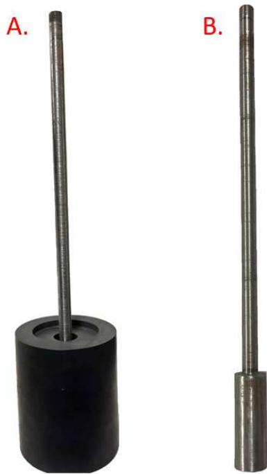
Figure 3: A) Alignment rod inside viscometer cup. B) Alignment rod.
