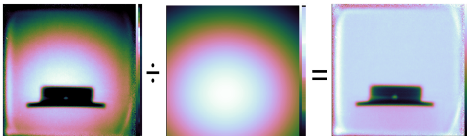
FIG. 6. Flattening procedure using the profile monitor data for the dynamic image from camera T. From left to right: the processed image containing the beam shape, the beam shape for this frame from the profile monitor data, and the image after dividing by the beam shape. The absence of the shape of the beam can be clearly observed in the final product.
