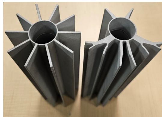
Figure 85: 3D-Printed Longitudinal Fin Tubes.
