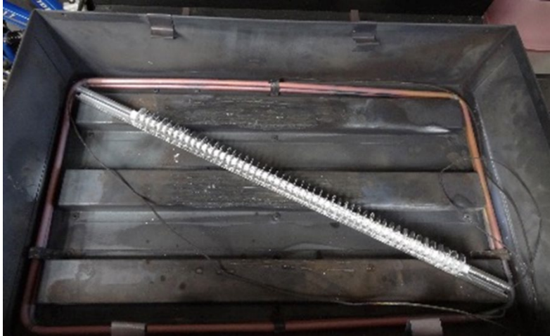
Figure 74: Optimized annular fin-tube assembly in brazing furnace.
