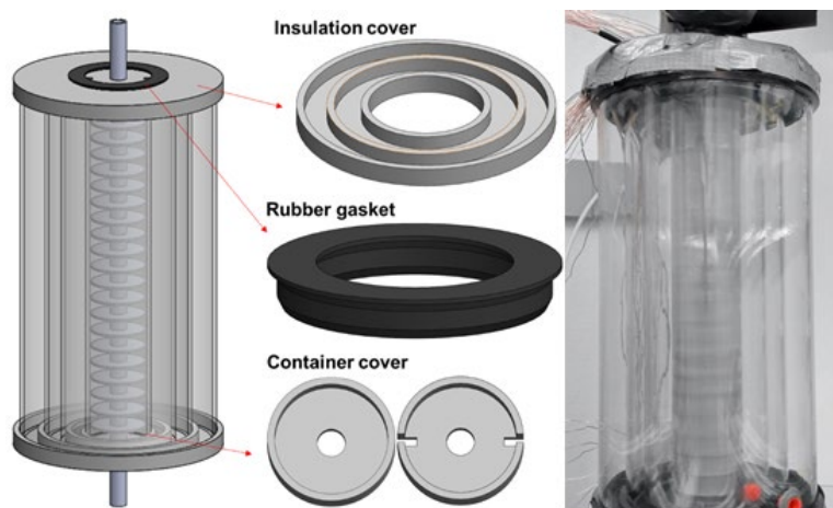
Figure 71: 3D-Printed Annular-Fin Tube PCM-HX Insulation cylinder assembly: (L) 3D model and (R) actual assembly.
