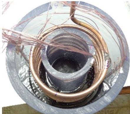
Figure 80: Helix Tube PCM-HX: Final assembly.
