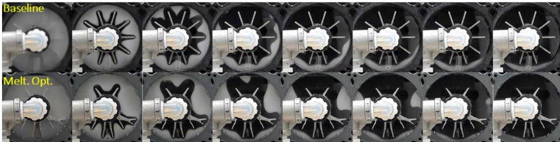
Figure 111: Images of melting fronts every 10 minutes
