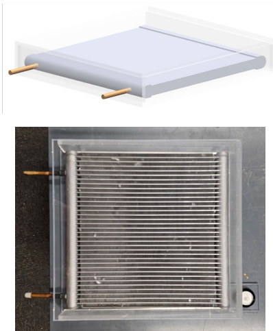
Figure 83: (TOP) Schematic view of Microchannel PCM-HX; (BOTTOM) Microchannel PCM-HX inside acrylic container.
