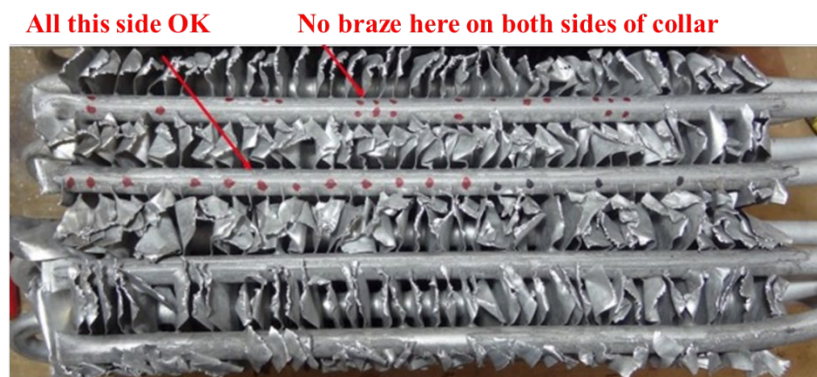
Figure 68: Dogbone-Fin HX Cut in Half (Post-Brazing).
