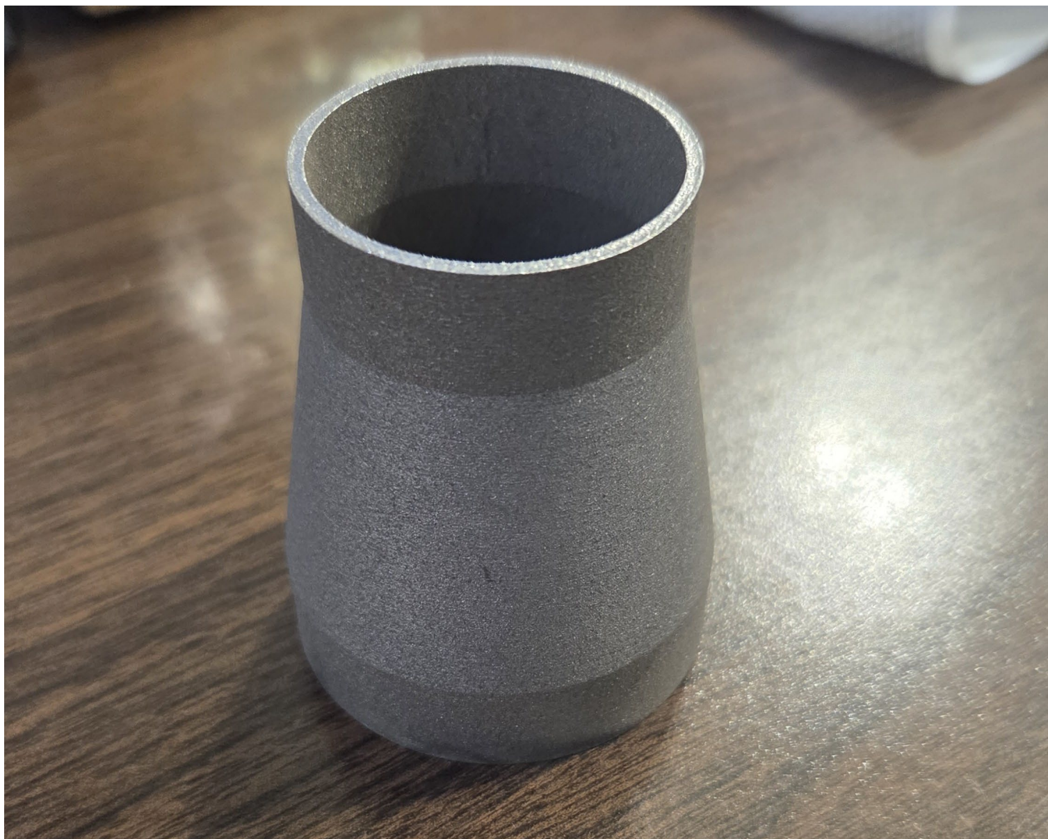
Figure 1: Control reducer being tested for outgassing is untreated. Made of 3d printed 316 steel.
