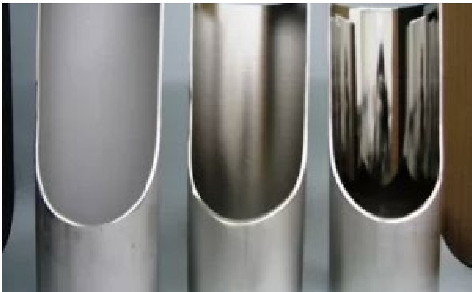
Figure 3: Example of the results of using electropolishing to polish parts. [1]
