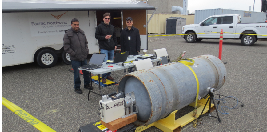
Figure 6. Picture shows the electrically cooled HPGe set up in location L3
