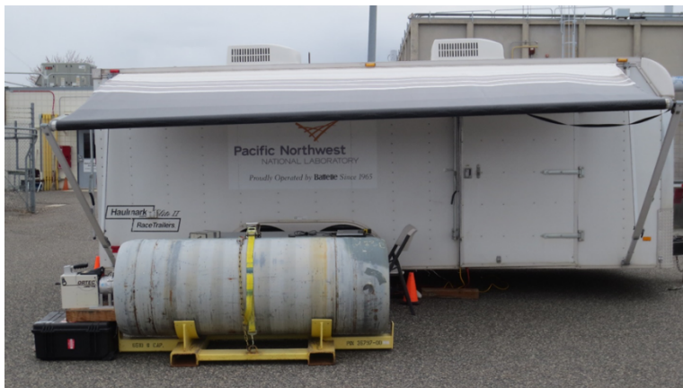
Figure 4. A 30B UF 6 cylinder located in place in front of the measurement trailer.
