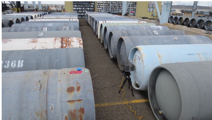
Figure 7. M400 CZT measurements in the Framatome cylinder yard
