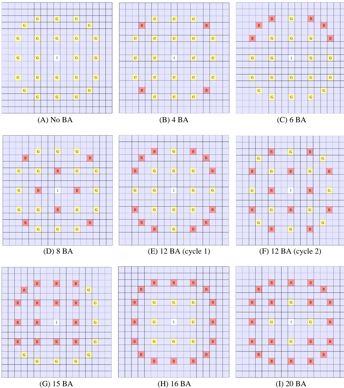
Figure 2.2. Fuel assembly configurations with burnable absorbers (B) and guide (G) and instrument (I) tubes.
