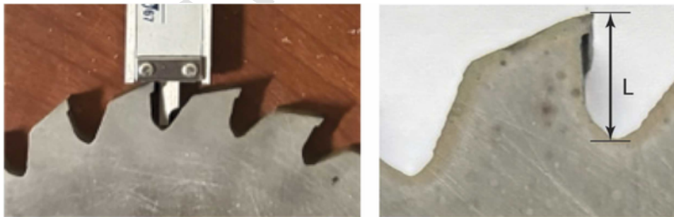
Fig. 4. Illustration of tooth length measurements where L is the length from the tooth base to the top edge.
