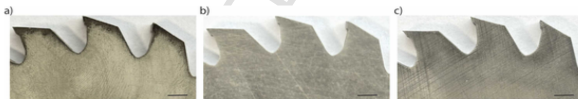
Fig. 6. Optical images of three cutters after completion of the shredder wear testing. (a) Borided D2, (b) D2, and (c) M42 cutters. Size of the scale bar is 5 mm.
