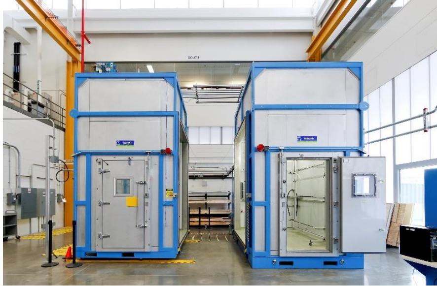
Figure 2. HAM chamber with indoor chamber (left) and climate chamber (right)
