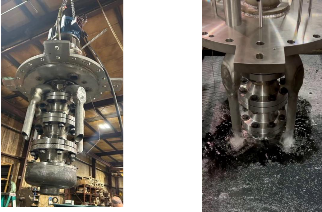
Figure 13. Lifting operating and water testing of the test rig by the subcontractor before the test rig was shipped to ORNL.
