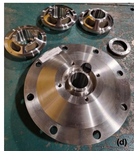
Figure 10. Fabrication progress of the (a, c) main mounting plate, (b) the bearing spider assemblies, and (d) the impeller offset outlet diffuser.
