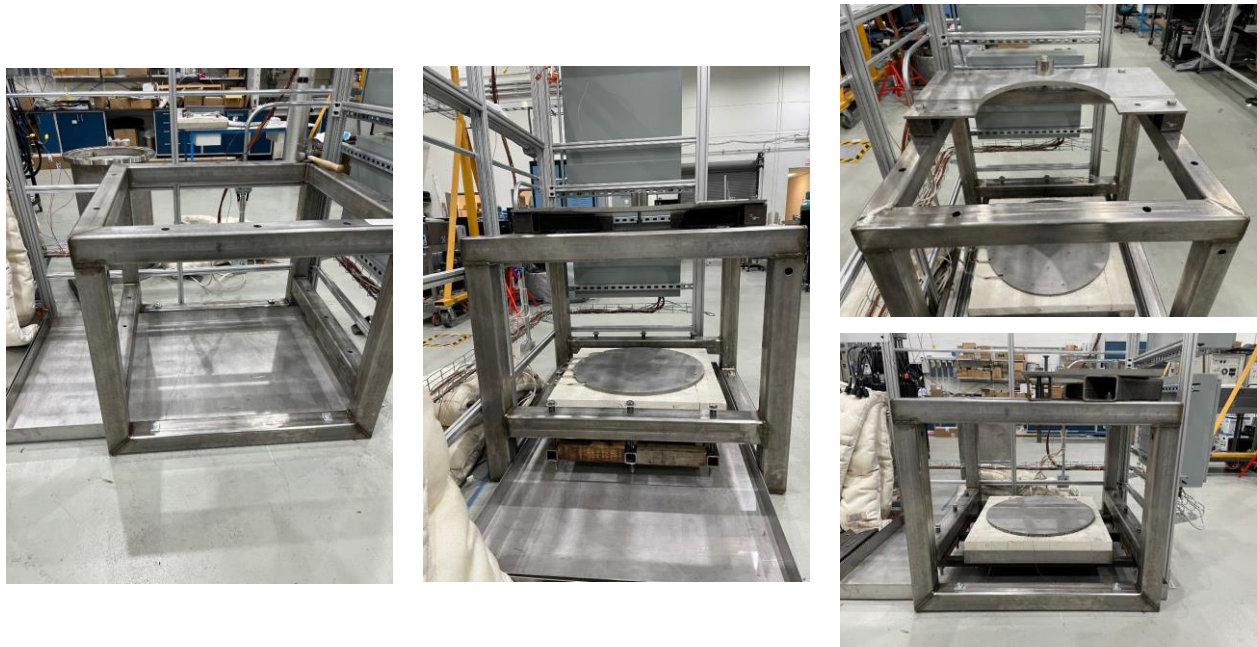
Figure 14. Frame, 2-piece plate, spring-loaded base, and drip trays of the support structure.
