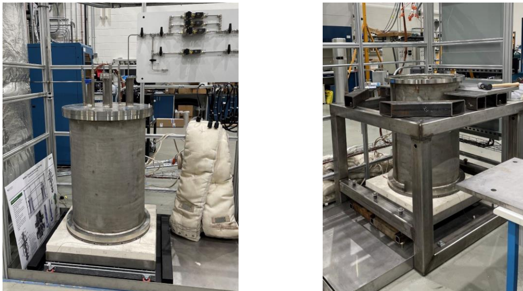
Figure 21. Installation of base plate heaters, tanks, and pump stand.
