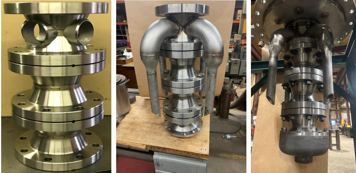
Figure 11. Fabrication progress of the column assemblies and return piping.
