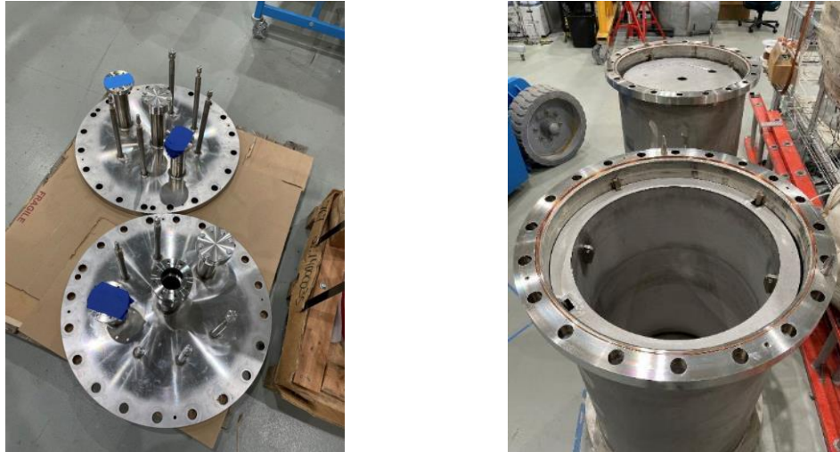
Figure 20. Lift and swap of existing Nickel 201 crucibles with new UNS S31600 variants. A new annular ring-type lid (right) was also fabricated to enable installation of the bearing test rig.
