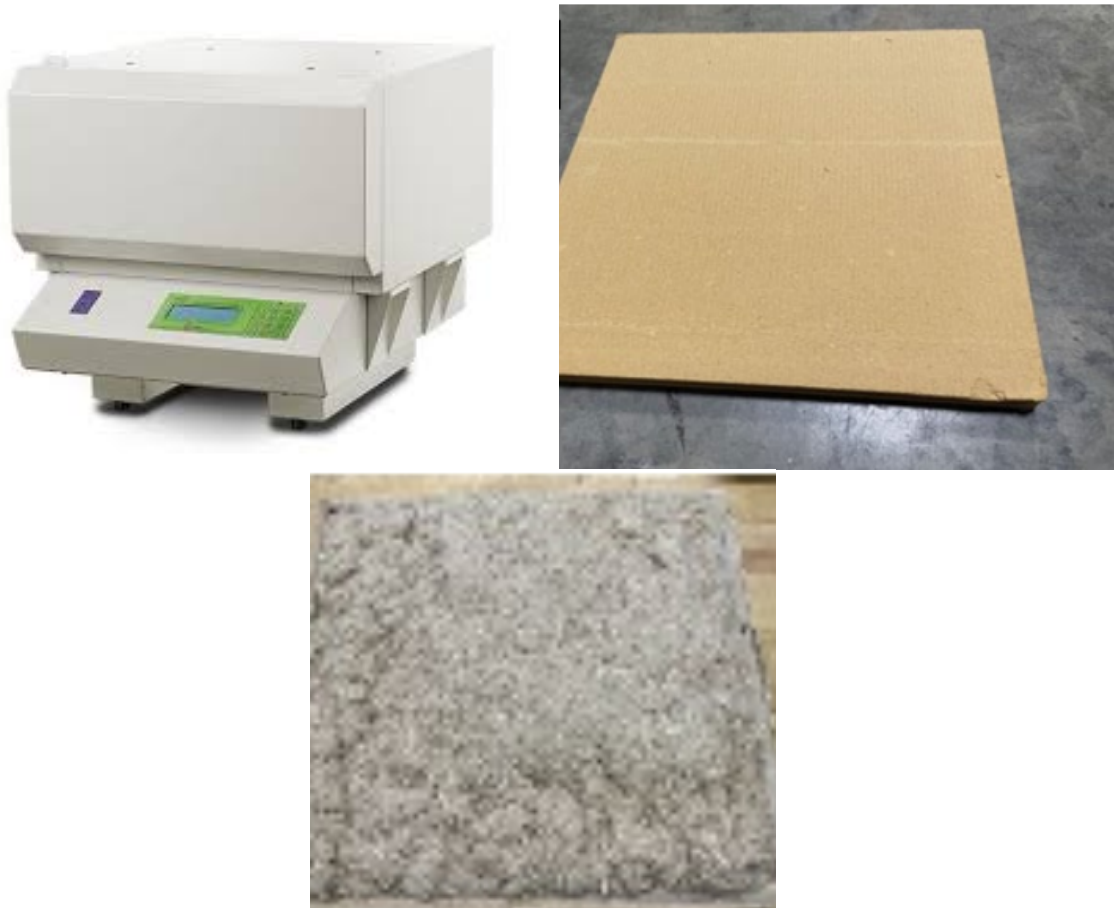
Figure 1. Heat flow meter and test specimen.
