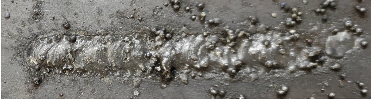
Figure 2: Initial testing of tungsten wire deposited on a mild steel substrate
