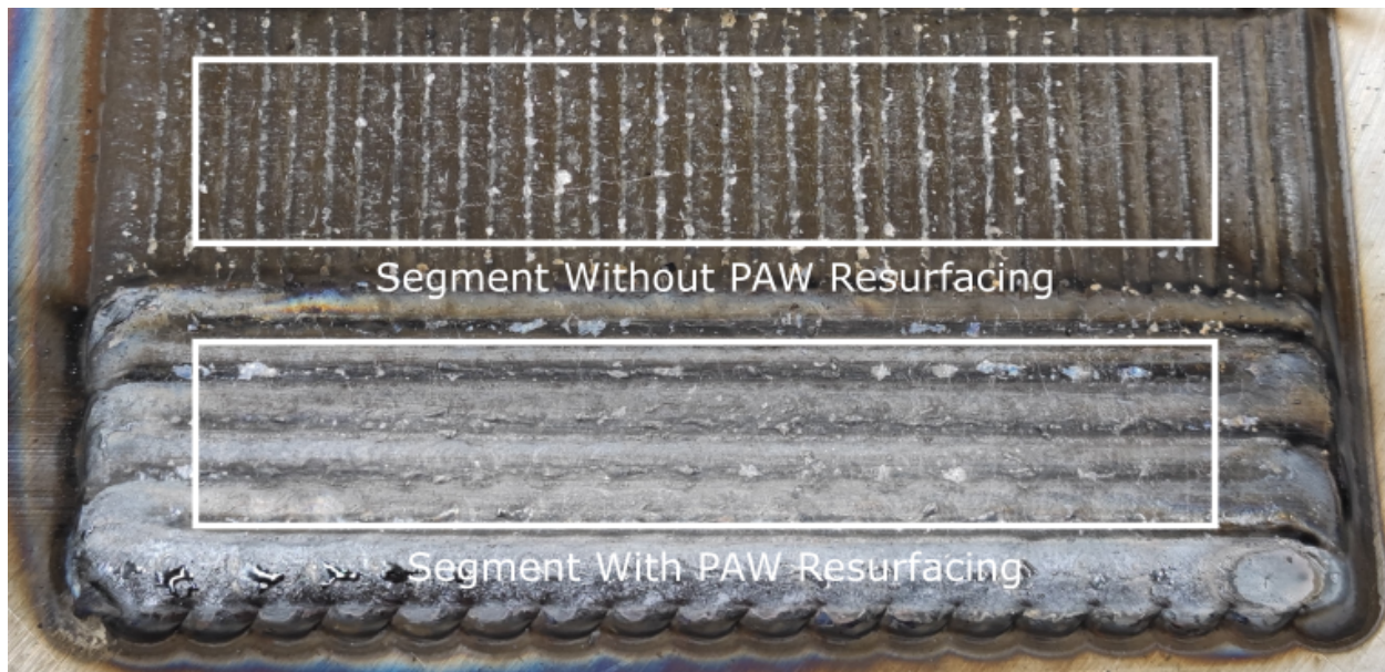
Figure 11: Beads that were initially deposited with the GMAW process are resurfaced with the PAW torch.
