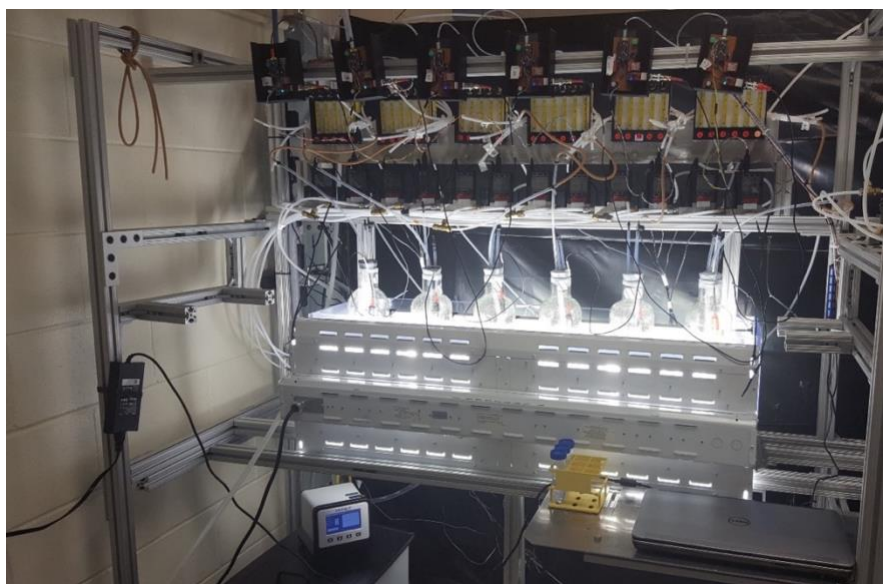
Figure 2-3. Setup used for the proportional CO 2 -controlled injection based on pH as well as CO 2 consumption monitoring. B/Cube function used to correct the pH by sending a voltage to the mass flow controller.
