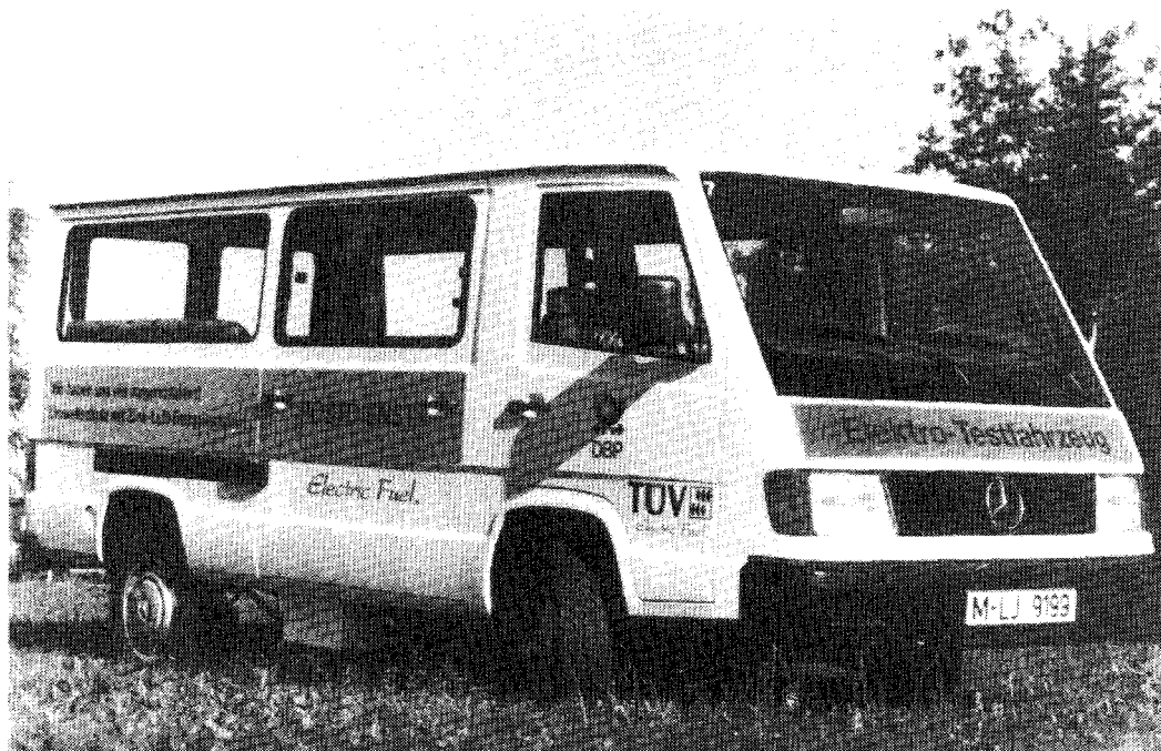
Figure 2. Mechanically Rechargeable Fleet Test by Postdlenst of Germany with Electric Fuel Battery.
