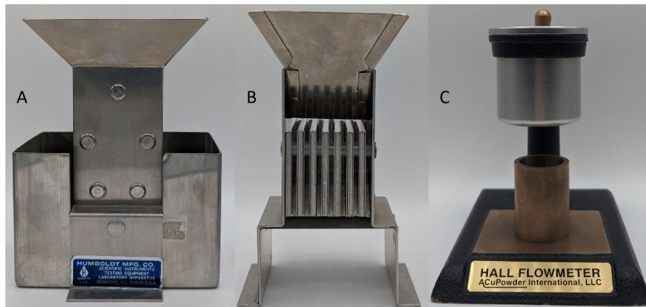
Figure 4: Powder splitter A) front view and B) side view and C) Hall-Flow Meter
