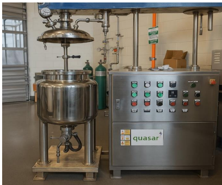
Figure 7.4.3: Pilot scale 100 L reactor for dark fermentation.
