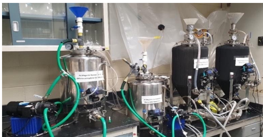
Figure 7.1.2: The left steel reactor is the microaerobic dark fermenter (DF), and the right steel reactor is the anaerobic DF, with the black reactors in the background being the anaerobic digestion inoculum reactors used for the initial DF reactor seeding.
