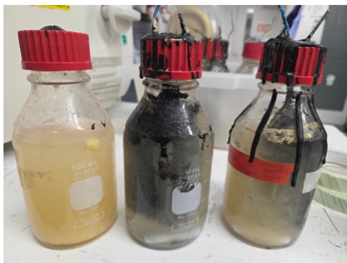
Figure 7.1.6. Image of MEC-fermentation reactors. Left to right: No electrode control reactor (NE), open circuit control reactor (OCP) and applied voltage reactor (MEC).
