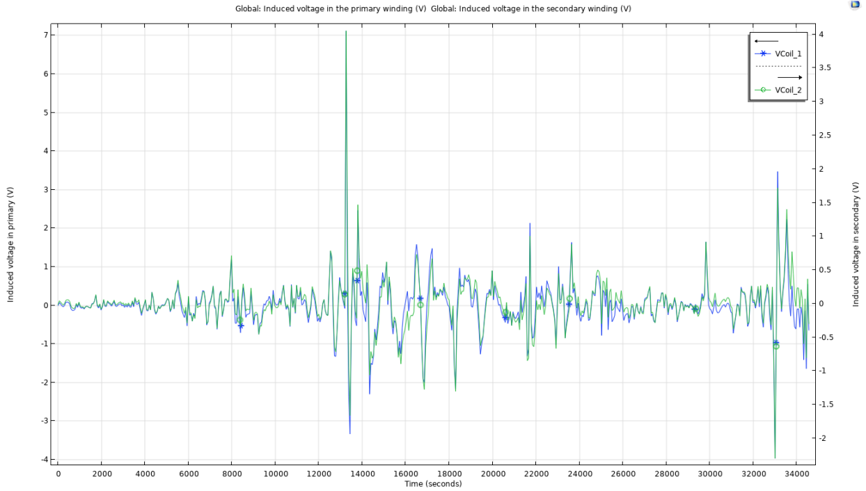
Fig. 14 Primary (blue) and secondary (green) voltages during GMD event. (Note: left y-axis indicates primary currents, while right y-axis indicates secondary currents).
