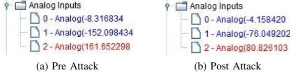
Fig. 6: Analog input signals from outstations in PASuite
