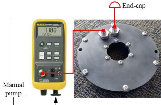
Figure 116: End-winding channel airtightness test setup
