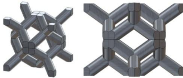
Figure 31: Dimetric and diagonal views of a rhombic dodecahedron-based unit cell
