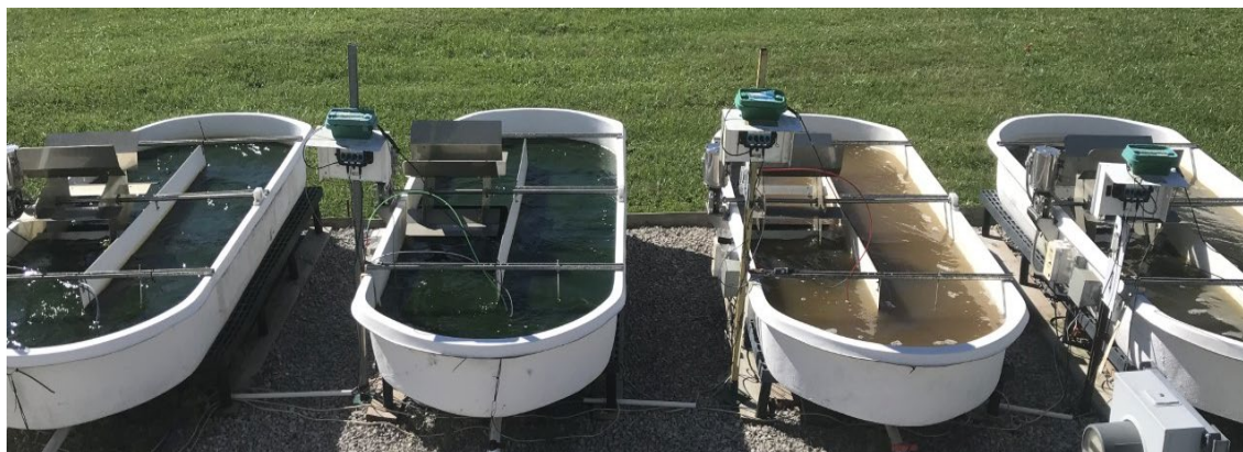
Exhibit 4.6.7. ORPs used for culturing experiments, 10 days after inoculation. Left: ORPs 1 and 2, fed with 10/1 \text{CO}_2/\text{NH}_3 ; right: ORPs 3 and 4, fed with pure \text{CO}_2 and \text{NaNO}_3 ; the cultures in ORPs 3 and 4 had crashed at this point. The \text{CO}_2 flow rate to each pond was 0.15 L/min.
