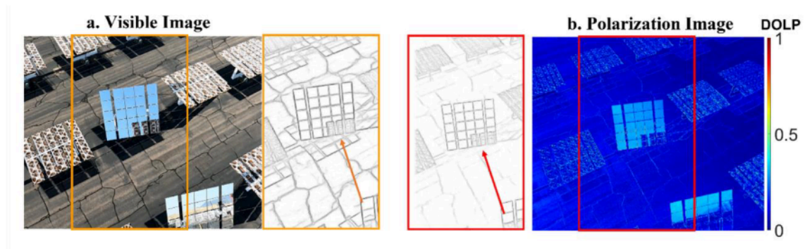
Figure 8. Example back-vs-ground scenario with the conventional image (left) and the degree of linear polarization image (right).
