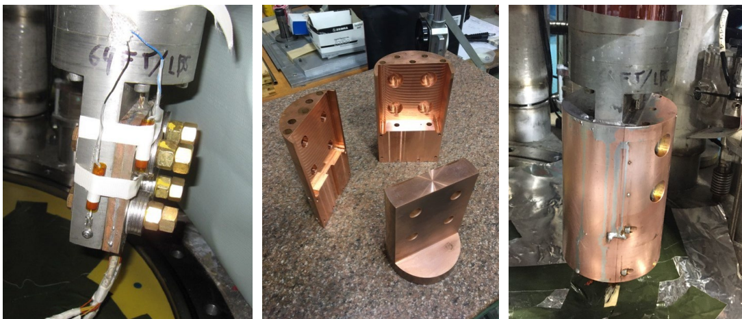
Figure 7. The left photo shows the original configuration, where a copper splice block containing the superconducting bus was bolted to the current lead bottom flag. The middle photo shows the new two-piece copper fixture with a current lead dummy flag used for testing. The right photo shows the copper fixture after being soldered onto the in-service current lead.
