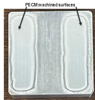
(b) specimen with textured surfaces that were processed using PECM
