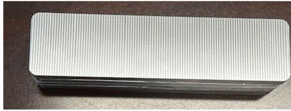
Figure 6.1.2 1:100 scale mold module flat (100 mm x 25 mm) ball nose end-milled surface
