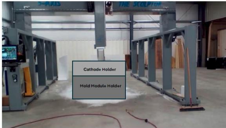
Figure 6.5.1 PECM cell within three-axis gantry system
