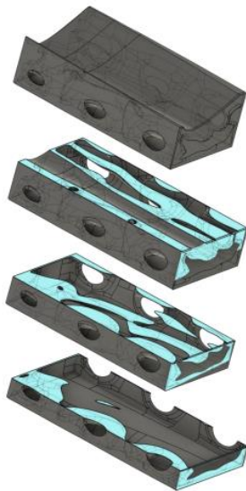
(c) section views of the mold module with air channels
