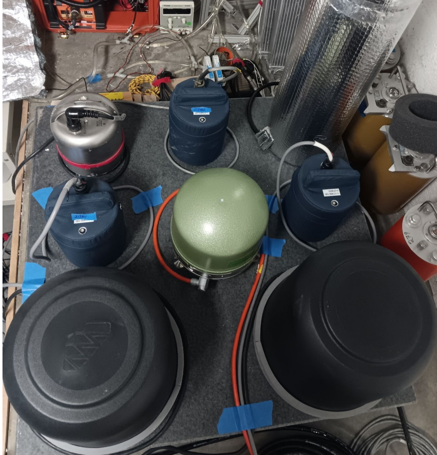
Figure 62 Sensors installed on seismic pier for self-noise test
