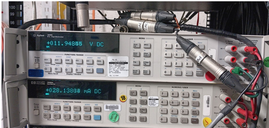
Figure 10 Power Consumption Configuration Picture
