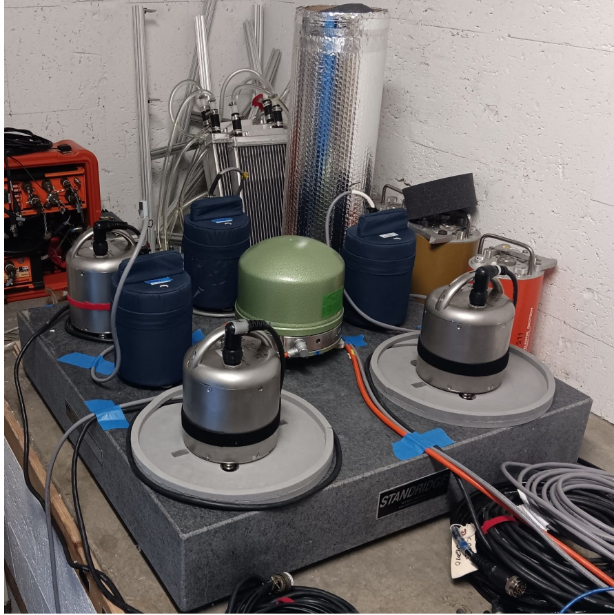
Figure 25 Sensors installed for Comparison Sensitivity Test
