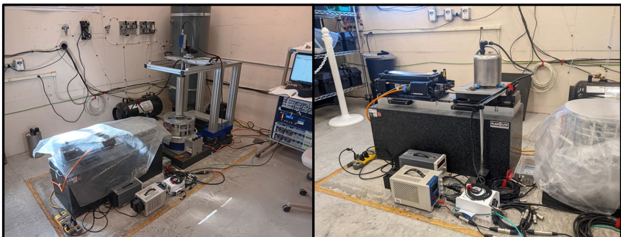
Figure 15 T120 Slim PH installed on vertical shake table (left) and T120 Horizon installed on horizontal shake table (right)
