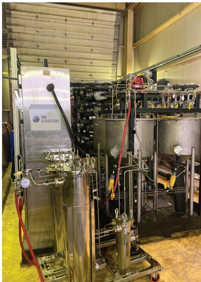
The Via Separations filtration skid enables black liquor concentration set up at the Ahlstrom-Munksjö Mosinee mill. Photo from Ahlstrom-Munksjö
