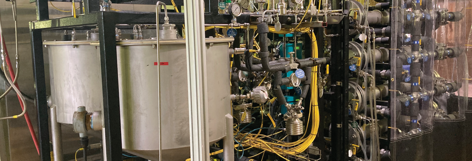
The Via Separations filtration skid enables black liquor concentration at a fraction of the energy required by the existing process. Photo from Ahlstrom-Munksjö
