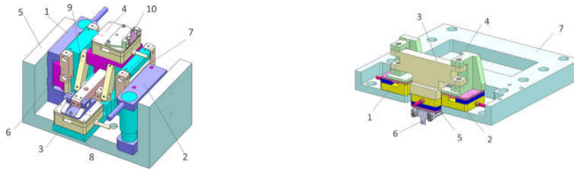
Figure 3. Left: A 3-D model of the nested flexural bearing structure for angular adjustments along the axes of XMLL1 and ZMLL1. The nested flexural bearing structure is operated by two PI™ M-110 motorized linear stages (1) and (2), and two PI™ M-663 PZT-driven linear stages (3) and (4). The linear stages (1) and (2) are mounted on a U-shaped base frame (5). Cooperated with the outer flexural bearing structures (6) and (7), linear stages (1) and (2) provide linear positioning in the Y direction and tilting adjustment around the X-axis for another U-shaped frame (8), which is the base for a 4-bar flexural bearing structure (9) nested in the outer flexural structure. The 4-bar flexural bearing structure is operated by the PZT-driven linear stage (3) to provide a precise angular positioning around the Z-axis. The linear stage (4), mounted on the top of the 4-bar flexural bearing structure, aligns the upstream MLL (10) in the X direction. Right: A 3-D model of the upper stages group, which includes three PI™ M-663 PZT-driven linear stages. A pair of linear stages (1) and (2) drive a carriage (3) through a set of flexural bearings (4) to perform linear positioning in the Z-axis direction with tilting adjustment around the Y-axis. The linear stage (5) provides the alignment in the X direction for the downstream MLL (6).
